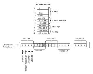
Fig. 2. Integer array chromosome encoding
