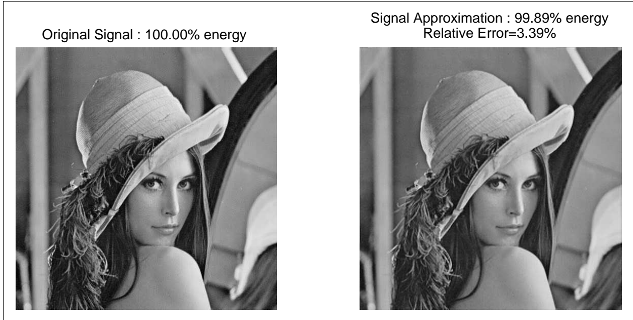
Figure 3.2: A side-by-side comparison of the original signal x and a reconstructed approximation using only the low-low frequency information in \hat{x} .
