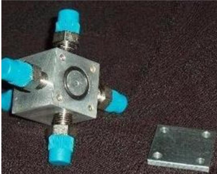
Figure 1-Co- axial Swirl Injector with Orifice plate
